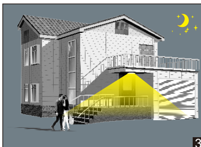
3 After moving sensor function start, if there is moving object around, the brightness of lamp be will be from 30% to 100%, and than keep 5 minutes.
